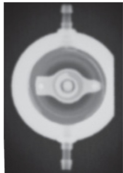
This proGAV valve is set at 11 cm H 2 O.
